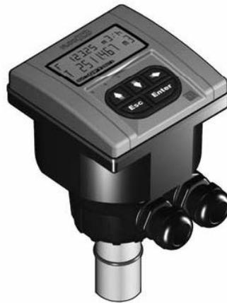
The FLOWX3 NEW F9.60M & F9.63M Insertion Magmeters are suitable to measure flowrate in both metal and thermoplastic pipelines. No moving mechanical parts and the high quality materials allow the measurement of liquids where suspended solids can be present or of abrasive liquids as long as they are conductive and homogeneous.
